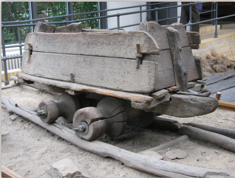
Early example of a Mine Tub on wooden rails at Siebenbürgen, 1890's. Note the use of rollers rather than wheels.
